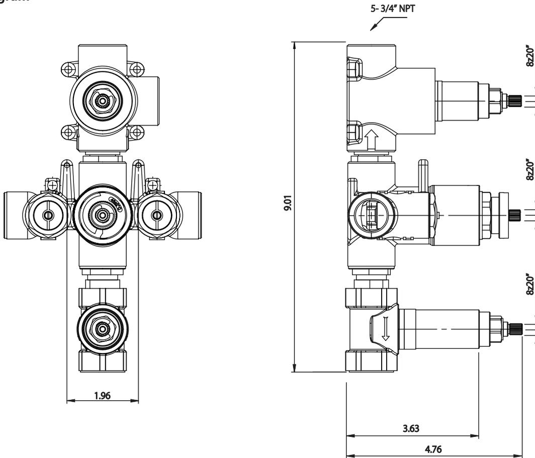
TVH.4501 | Three Output 3/4" Thermostatic Valve Page 2 of 2
